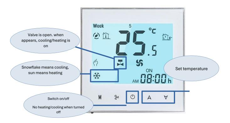
The current temperature is shown on the display in idle state, the desired temperature is only visible during adjustment. By pressing the arrow keys, you can set the desired temperature with an accuracy of  $0.5\,^{\circ}$ C.
